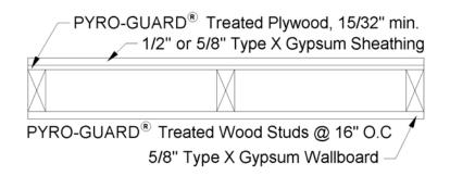
INTERIOR SIDE: One layer <sup>5</sup>/<sub>8</sub> inch type X gypsum wallboard or water resistant backer board or veneer base applied parallel with or at right angles to studs fastened with GWB-54 nails at 8 inches o.c. or 8 inches o.c. on the edges and double nailed in the field at 12 inches o.c. or 1 <sup>1</sup>/<sub>4</sub> inch Type W drywall screws at 16 inches o.c..
