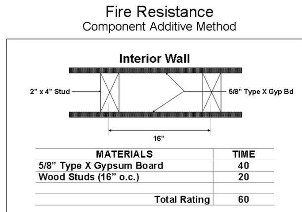
Figure 1. Interior wood stud wall of Example 1
