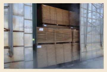
Kilns are used for drying lumber and plywood after treating. Carefully removing water from the wood results in consistent, high-quality FRTW.
