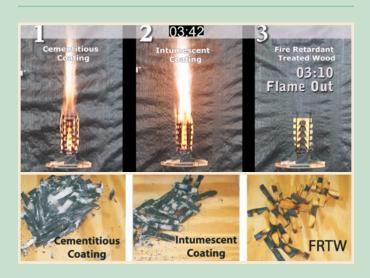
As the ASTM E160 test demonstrates, FRTW self-extinguishes when the burner is removed at 3 minutes. Coated wood does not self-extinguish and continues to burns until it is completely reduced to nothing but ash and coating residue.
