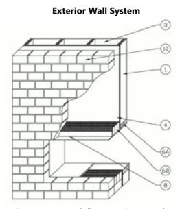
1. **Framing Members (CIKV, BPVV)\*** — Pressure-treated, fire-retardant wood studs, nominal 2 by 4 in., spaced 16 in. (406 mm) OC effectively firestopped. As an alternate, pressure-treated, fire-retardant wood studs, nominal 2 by 6 in., spaced max 24 in. (610 mm) OC, effectively fire-stopped. Additional studs to be used to completely frame window openings (see Item 6).
